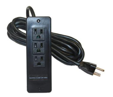
The three inline outlets power bar model **SF-PB3** accepts standard power cords with a 3rd outlet for oversized plug-in/transformer to accommodate cell phones and PDAs. It includes three grounded outlets. It has a 12 AMP rating and a 10 ft. 14-3 gauge power cord. The unit mounts in a  $5-1/4" \times 1-7/8"$  cutout. (Same cutout as PC-PATCH)
